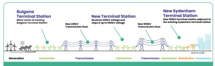
New overhead double circuit 220kV transmission line between the existing Bulgana Terminal Station and a new terminal station to the north of Ballarat. From there to the proposed terminal station at North Sydenham, a new overhead double circuit 500kV high voltage transmission line will be required.\*
