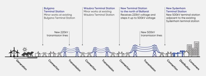
New overhead double circuit 220kV transmission line between the existing Bulgana Terminal Station, connecting to the existing Waubra Terminal Station and a new terminal station to the north of Ballarat. From there, a new overhead double circuit 500kV transmission line connecting to a new terminal station at Sydenham.
