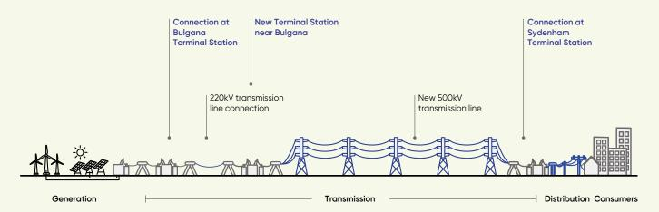
Proposed overhead 500kV double circuit transmission line from Bulgana to Sydenham
