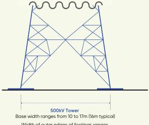
Width of outer edges of footings ranges from 12 to 20m (18m typical)
