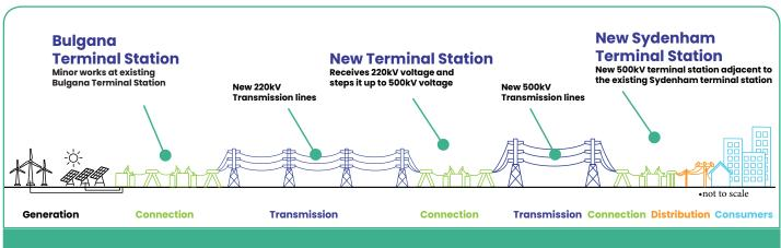
New overhead double circuit 220kV transmission line between the existing Bulgana Terminal Station and a new terminal station to the north of Ballarat. From there to the proposed terminal station at North Sydenham, a new overhead double circuit 500kV high voltage transmission line will be required.\*
