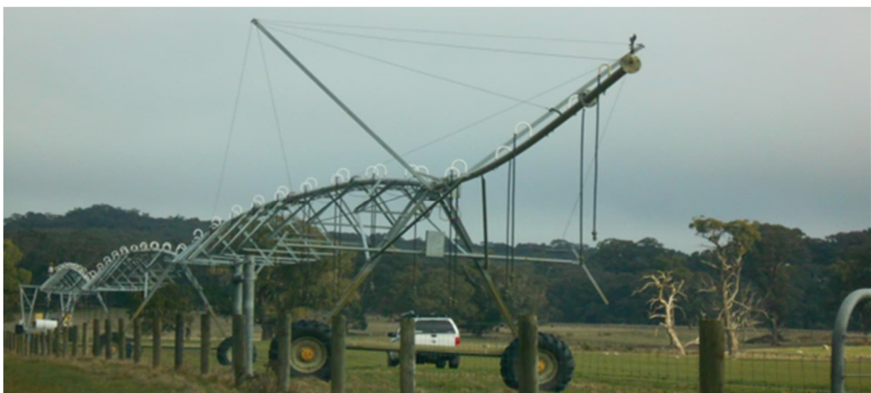
Figure 6-10: Centre pivot irrigator with 'rabbit ears' and end gun (Source: Central Highlands Water)
